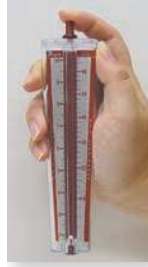
For high scale reading, finger covers hole
