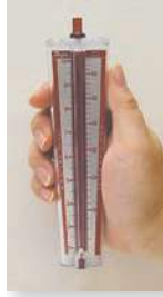
Hold this way for low scale reading
